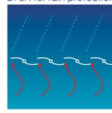
With louvres opened a small distance, protection is still provided for light rain.
